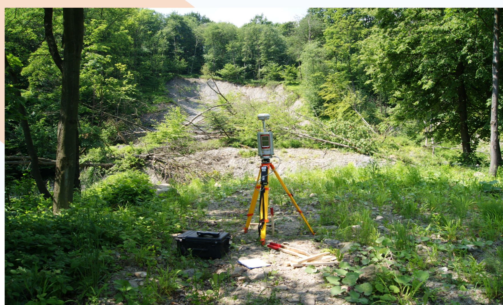
Fig. 1. Terrestrial laser scanning position of the landslides source: Jarosław Cebulski
