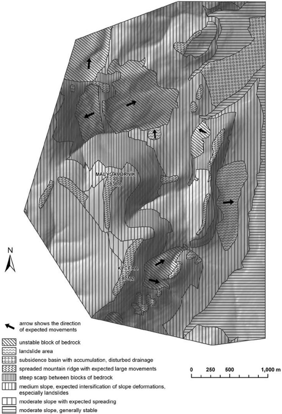
Fig. 7. Digital engineering-geomorphological 3D model of expected terrain deformations and geohazards in relation to planned deep mining of black coal in the western part of the Trojanovice mine area derived from the digital geomorphological map
