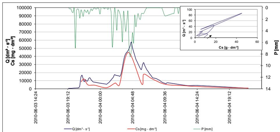
Fig. 6. Sediment concentration during the flood in June 2010 and the hysteresis.
