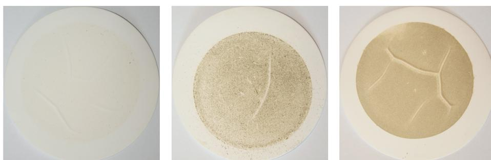
Fig. 3. Drains after filtration; W-1 – upper lake, small amount of suspended load, W-8 – talus cone, fine sand fraction, W-9 – talus cone, mud fraction
