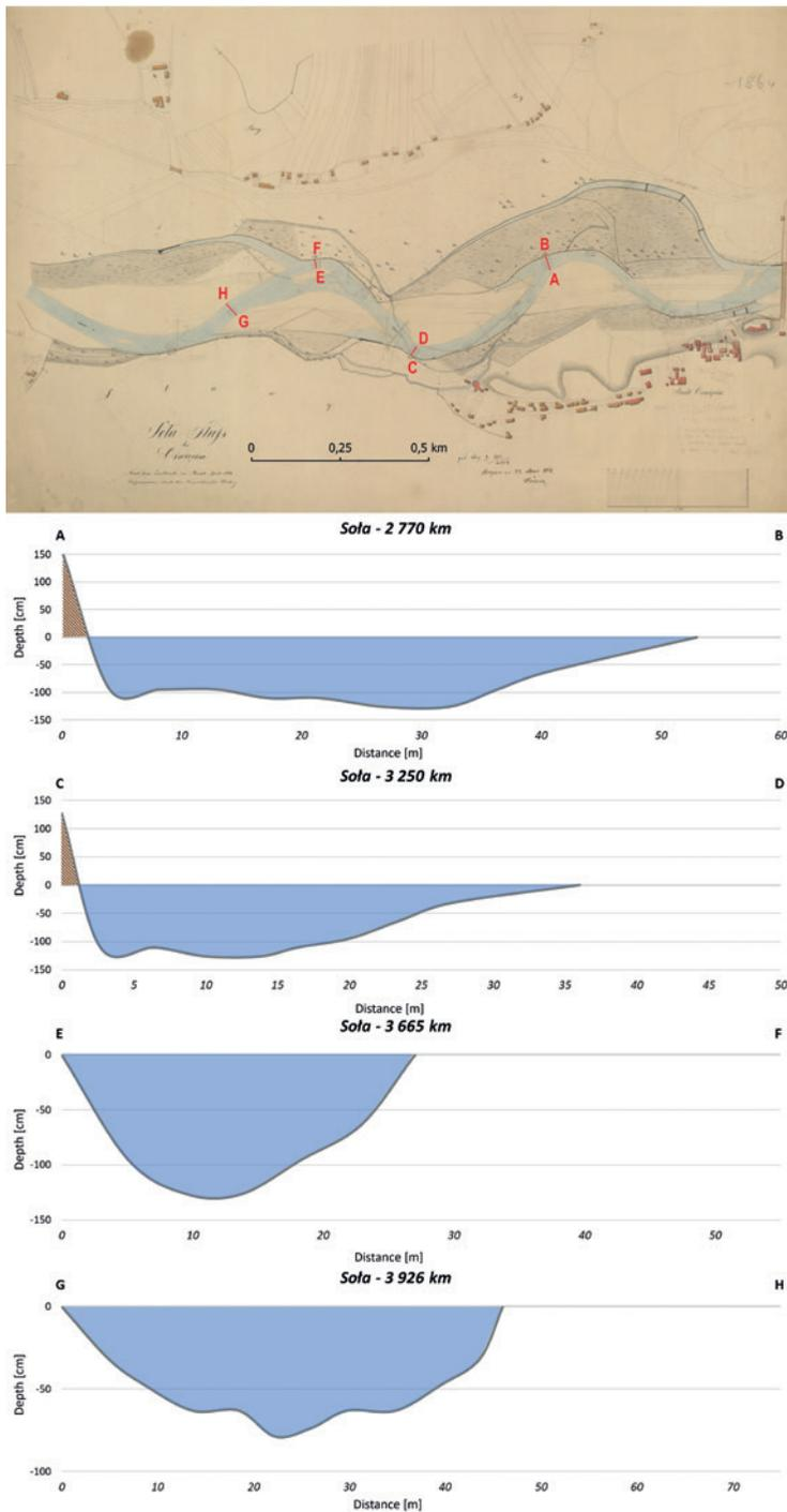
Fig. 8. Map from 1864 of the Soła channel in the Oświęcim area and cross section of the Soła channel (Soła Fluß bei Oświęcim..., 1864)
