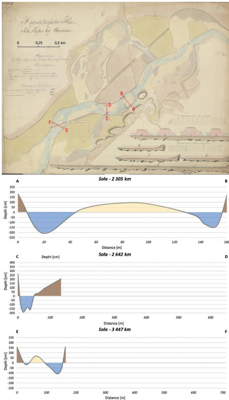
Fig. 4. Map from 1812 of the Soła channel in the vicinity of the town of Oświęcim and cross section of the Soła channel (Hydrotechnischer Plan..., 1812)
