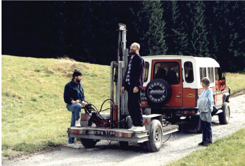
Photo 2. Impulsive source with acceleration EWG-III (BISON Inc.) used in the field for generating seismic waves (Photo A. Kotarba)
