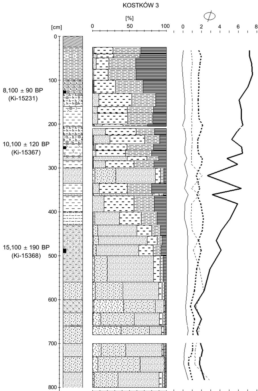
Fig. 6. Lithological sequence, grain size indices and radiocarbon datings of the Boreal paleochannel in the Kostków 3 borehole log. Explanation see Fig. 3
