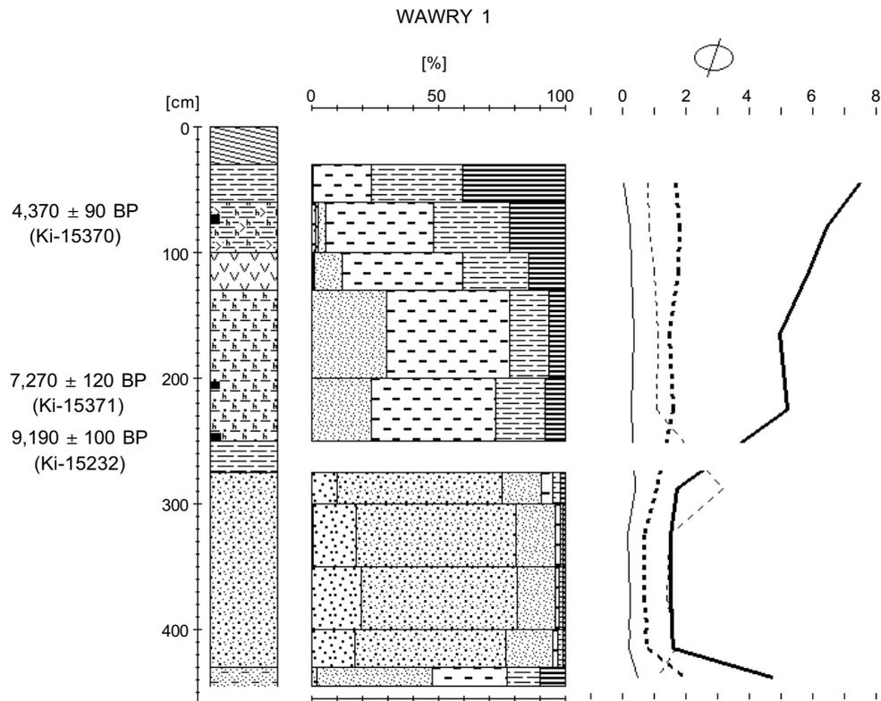
Fig. 5. Lithostratigraphical sequence and grain size indices of the Preboreal paleochannel in the Wawry 1 borehole log. Explanations see Fig. 3
