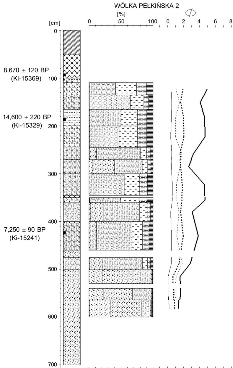
Fig. 4. Lithostratigraphical sequence and grain size indices of the Younger Dryas/Preboreal paleochannel in the Wólka Pełkińska 2 borehole log. Explanations see Fig. 3
