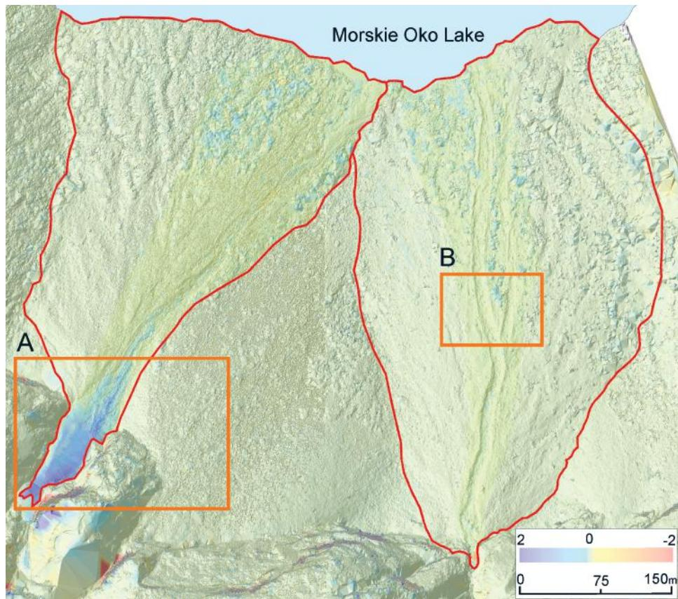
Fig. 6. DoD model of the studied talus cones surfaces for period 2011–2013. Rectangles A and B mark fragments of the talus cones shown in details on Figure 7.
