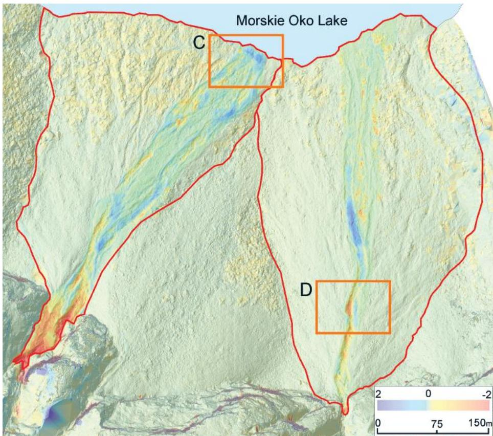
Fig. 7. DoD model of the studied talus cones surfaces for period 2013–2017. Rectangles C and D mark fragments of the talus cones shown in details on Figure 8.
