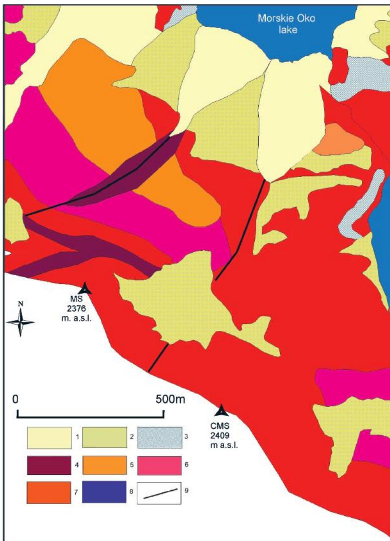
Fig. 2. Geological sketch of the study area. 1 – loamy-sandy-stony to boulder sediments of talus-alluvial cone, 2 – loamy-sandy-stony to boulder sediments of talus cone, 3 – moraine deposits, 4 – mylonites and cataclasites, 5 – granites with pegmatites and aplites, 6 – granites with K-feldspars, 7 – granodiorites and tonalites, 8 – lakes, 9 – faults
