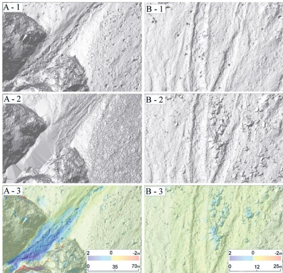
Fig. 8. Detailed digital terrain models and DoD model of the talus cones fragments marked at Figure 5. The Szeroki Piarg: A-1 – 2011, A-2 – 2013, A-3 – DoD; the Zielony Piarg: B-1 – 2011, B-2 – 2013, A-3 – DoD.
