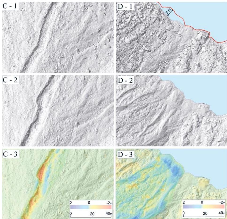
Fig. 9. Detailed digital terrain models and DoD model of the talus cones fragments marked at Figure 6. The Szeroki Piarg: C-1 – 2013, C-2 – 2017, C-3 – DoD; the Zielony Piarg: D-1 – 2013, D-2 – 2017, D-3 – DoD.
