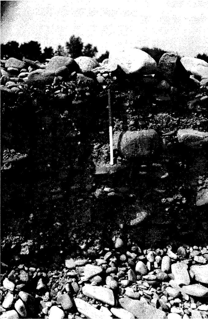
Photo 1. Structure of sediments forming the longitudinal gravel bar. Note that deposits are of very non-uniform grain-size. Pavement layer is clearly differentiated from underlying sediments both by grain-size and sorting. Scale is 20 cm
