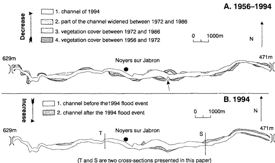
Fig. 7. Evolution of the channel in the Jabron flood plain. A — between 1956 and 1994 before the 1994 flood; B — after the 1994 flood drawn from aerial photographs. T and S are the two cross-sections of Figs 5 and 6
