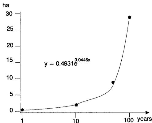
Fig. 10. Model of channel surface increase in relationship with flood frequencies
