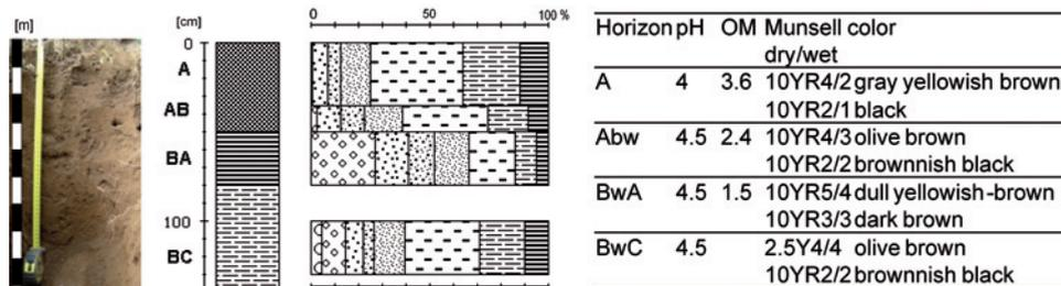
Fig. 5. Properties of soil profile DA2. (Grain size composition see Fig. 4)
