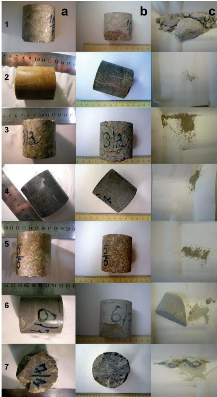
Fig. 10. Conditions of selected rock samples: a) before weathering simulation, b) after completion of frost weathering simulation, c) picture of the result of weathering; 1 – dolomite breccia, 2 – quartzite sandstone, 3 – white granite, 4 – amphibolite, 5 – brown granite, 6 – fine-grained conglomerate, 7 – organodetrital limestone
