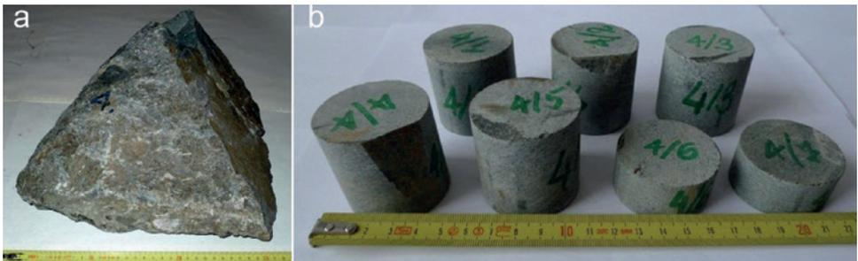
Fig. 3. Block and cut-out rock samples, for simulation of weathering and strength tests, on the example of sample no. 4. a) rock sample before core cutting, b) rock sample after core cutting
